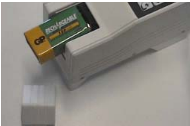
Figure 7. Accumulator compartment open.
